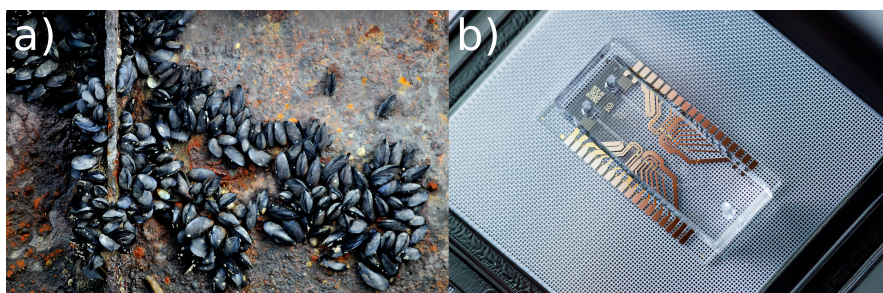
Figure 1.1: a) : Marine organisms growing on ships can cause environmental and economic damage. Anti-fouling brush coatings have been proposed as a solution. Image by Luis Bartolomé Marcos released under CC-BY-SA 4.0 International license b) : A microfluidic chip. Responsive polymer brushes can be used as a tool to control the flow of liquid through the channels on such chips. Image by FMN Laboratory, Bauman Moscow State Technical University released under CC-BY-4.0 International license.
