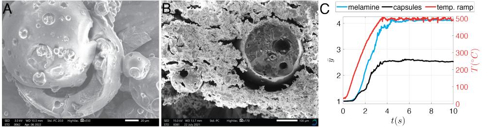
Figure 1.4: Scanning electron microscope images: A) A sliced microcapsule. B) Microcapsule embedded in the water-based intumescent coating. C) A plot of the average expanding front normalized by the initial thickness of the intumescent coat over time with different blowing agents.
