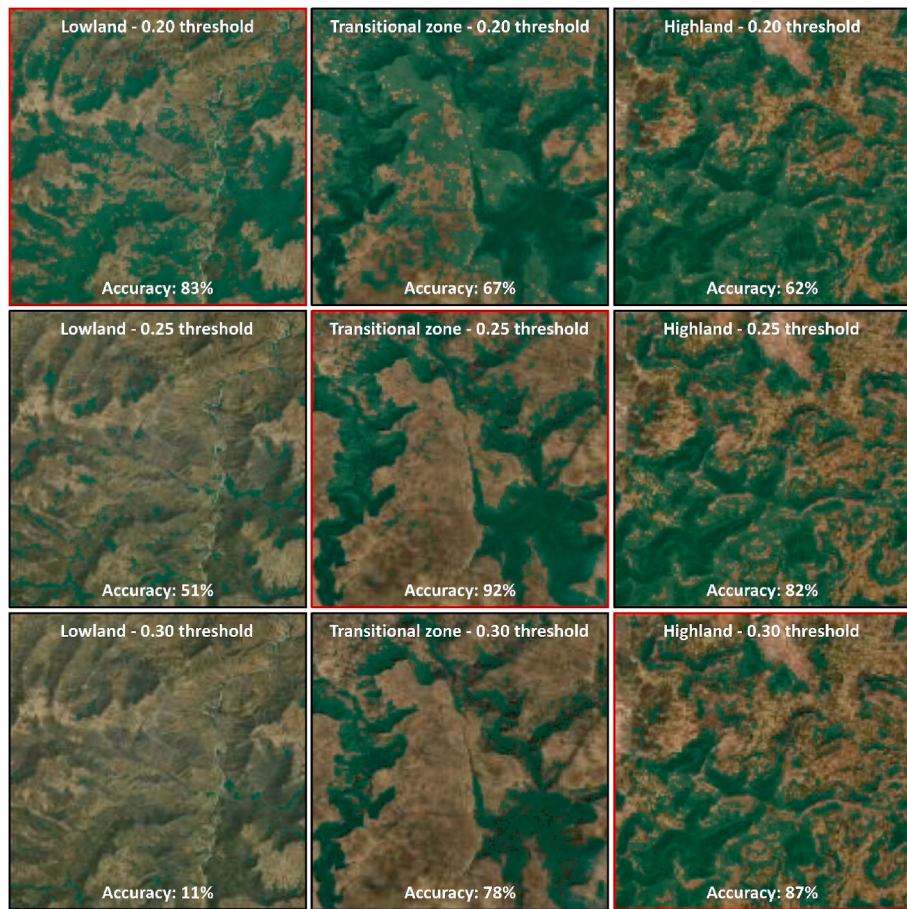
Fig. 2. NDVI thresholds to detect woody vegetation cover at different heights, where different vegetation types are found at various compositions. Best fitting threshold values are highlighted in red based on their performance accuracy indicated in percent. (For interpretation of the references to color in this figure legend, the reader is referred to the Web version of this article.)
