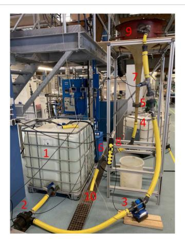
**Figure 4: Photo of the large funnel setup.** (1) Groundwater reservoir; (2) water pump; (3) water flow meter; (4) syringe with tracer; (5, 6) glass adapters with the oxygen sensor spot; (7), (8) pH probes; (9) Schauberger hyperbolic funnel; (10) water drain. Please click here to view a larger version of this figure.
