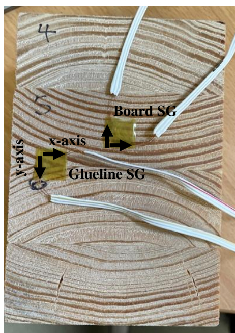
Figure 5: Strain gauge positioning on samples.
