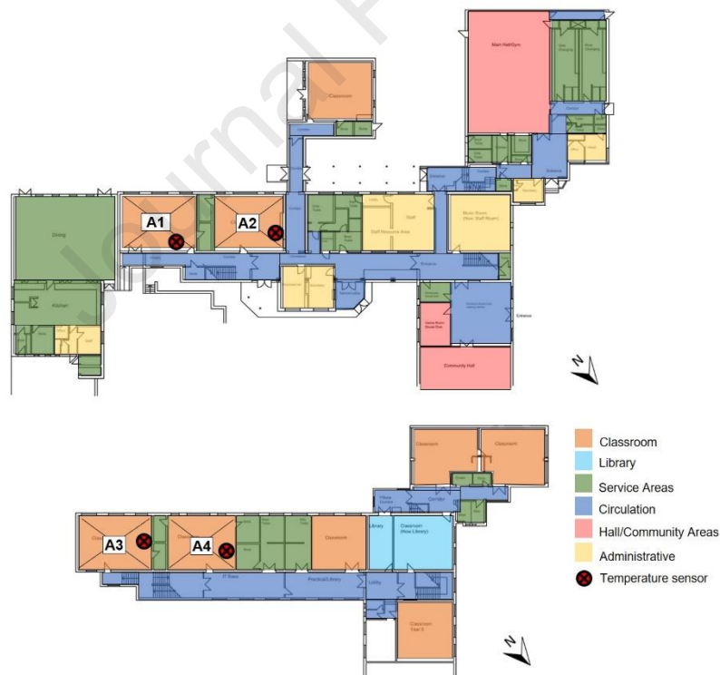
Figure A.1. Floor plan of School A. (up: ground floor, down: first floor)
