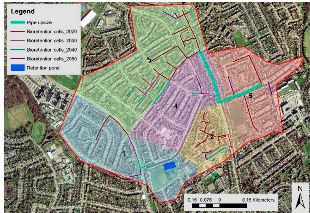
Figure 3. Proposed implementation location of the selected blue-green and grey infrastructure options in the study area (Contains Ordnance Survey data (2020)).
