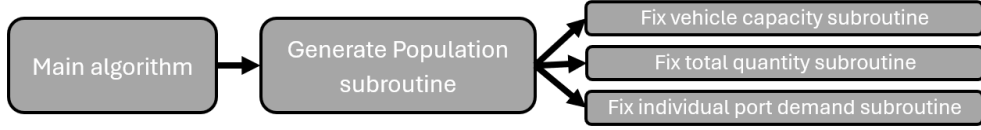
Fig. C1: Main algorithm and subroutines connections.
