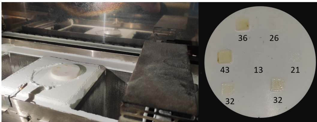
Figure 6.15: Sintering of PA12 particles at the surface of PA12-paraffin compacted disks for different powder-velocity ratios using the Sharebot SnowWhite SLS 3D printer. The numbers indicate the power-velocity ratio in Ws/m used to produce 5x5 mm squares with a hatch spacing of 0.1 mm.
