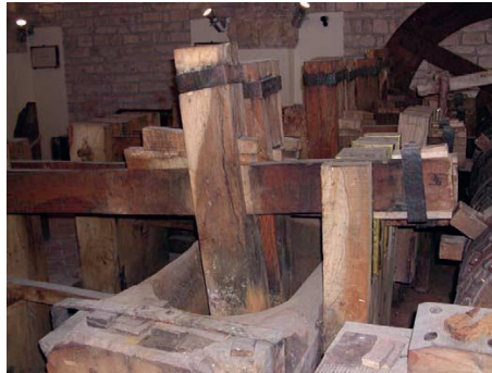
Figure 2.2 Picture of wooden stamper. Driven by a watermill. [73]
