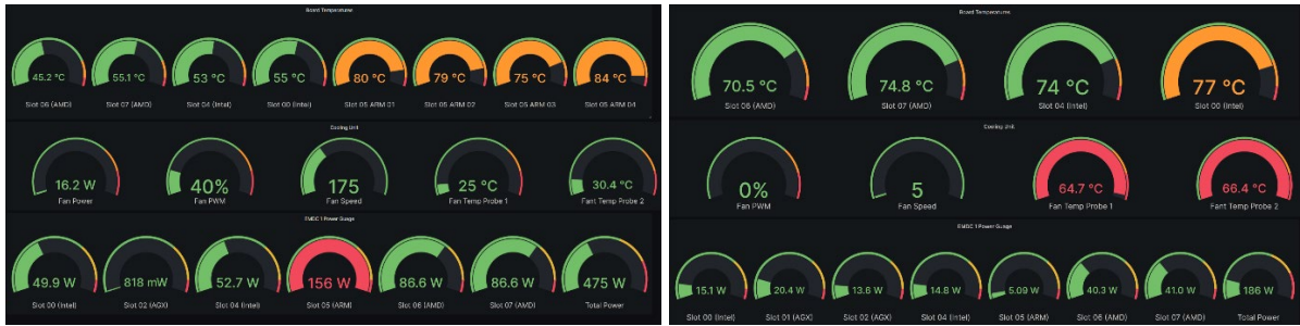
Figure 4. Left: Test results with fan set at 40% of PWM to operate all nodes without any throttling for PUE = 1.034; Right: Test results with ARM off and fans off...completely passive cooling.
