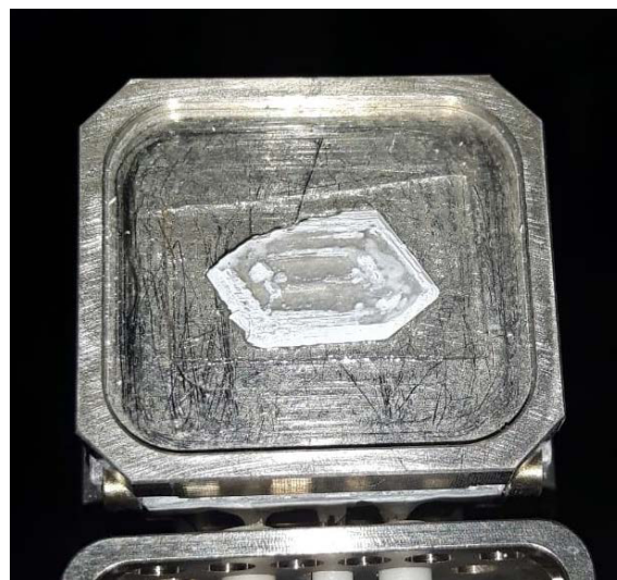
Figure 10. XRD measurement of a fresh single crystal, together with the identifiable crystallographic planes. The peaks originating from the dense potassium carbonate layer are denoted as the KC layer with Miller indices ( hkl ). The water plane with Miller indices represents the plane almost perpendicular to the KC plane. The photograph shows the placement of the single crystal in the XRD sample holder looking onto the (020), (040), and (060) planes.
