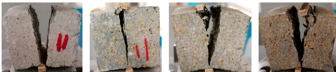
Fig. 28. Fracture pattern of print samples tested in u direction for splitting tensile stress. (a) Reference mix; (b) CR51 mix; (c) CR67 mix; (d) CR100 mix.
