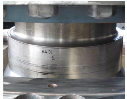
c) Appearance of mechanical damages in area 3
