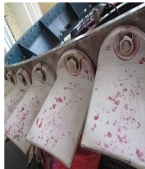
Figure 4. Appearance of mechanical damages detected at the upper and lower row of the ventilation ring vanes
