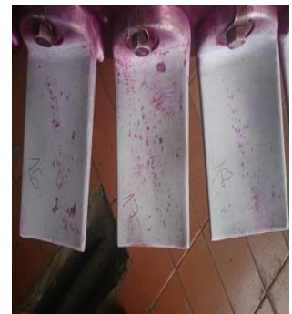
Figure 4. Appearance of mechanical damages detected at the upper and lower row of the ventilation ring vanes
