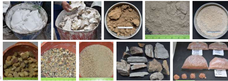
Fig. 1 Raw materials used during the design of conservation mortars (Photo-documentation of the MoDeCo2000 project)
