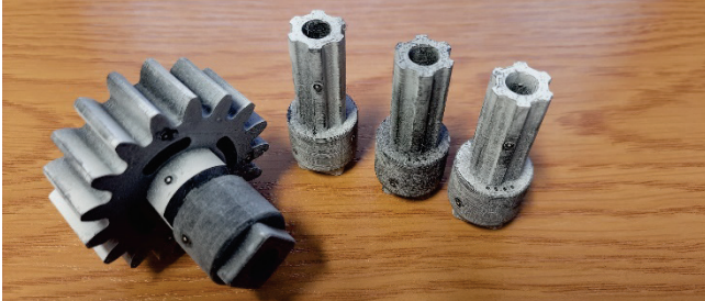
Figure 25 Checking the correctness of the prototypes geometry made using the FFF method
