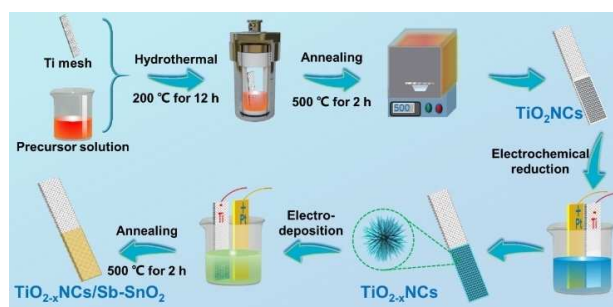
Figure 1. Preparation procedures of the TiO 2-x NCs/Sb–SnO 2 electrode.
