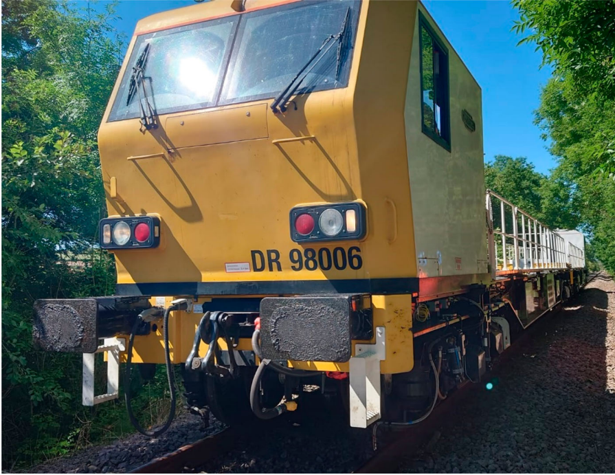
Figure 1. MPV with instrumented car nearest the camera.
