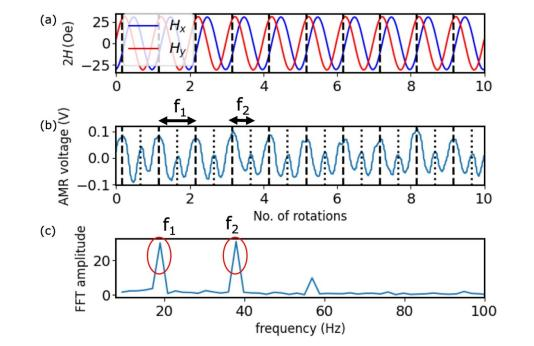
**Figure 4.** (a) The  $H_x$  and  $H_y$  components of the field profile that was applied to the sample and (b) the measured AMR signal for the first 10 rotations. (c) The Fourier transform of the signal with the  $f_1$  and  $f_2$  components marked.
