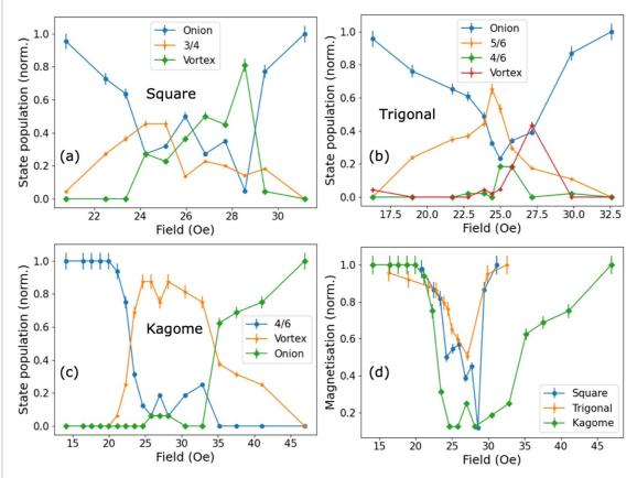
**Figure 3.** The magnetic state populations for the (a) square, (b) trigonal and (c) Kagome lattice NRAs as  $H_{rot}$  is varied. The magnetic states are schematically shown in figure 2. (d) The variation of the net magnetisation along the saturation direction with  $H_{rot}$  for the three lattice arrangements.
