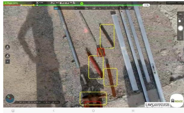
Fig. 6. Corrosion detection of pipes during the trials at PPC premises.
