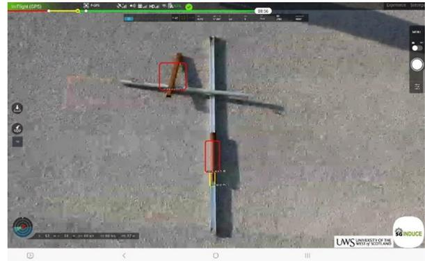
Fig. 5. Corrosion detection of pipes during the trials at PPC premises, with corroded ones overlaps with not corroded.
