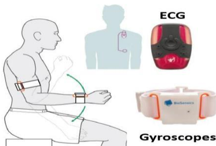
Figure 1: Wearable devices (gyroscopes) to obtain angular velocity and ECG during the UEF physical task.
