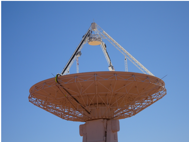
Figure 1. A 12-m ASKAP antenna, equipped with a Mark-II Phased Array Feed – Photo Credit: Robert Hollow, CSIRO.
