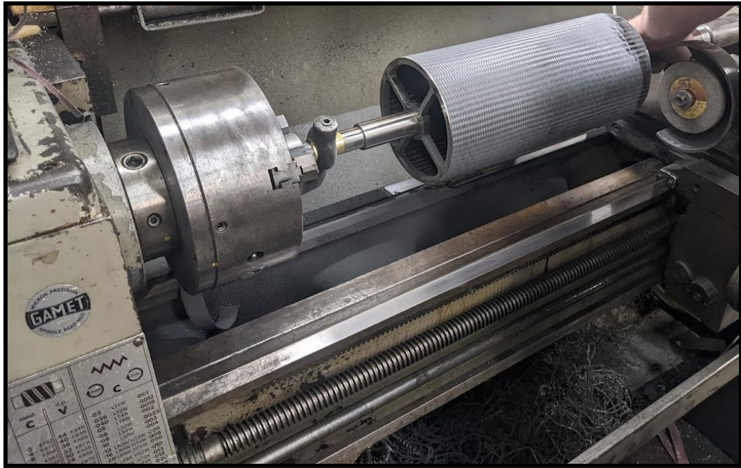
Figure B3: Upgraded idler roller after precision surface grinding
