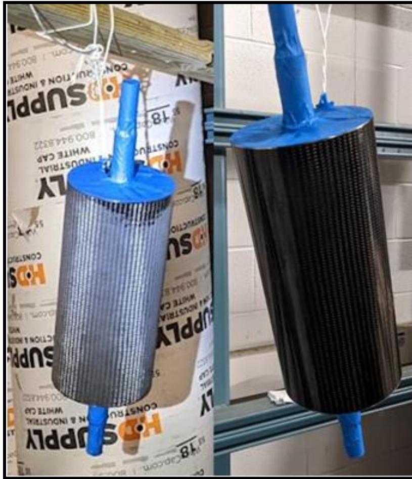
Figure B4: Final coating of idler roller CRFP body with acrylic resin based clear coat
