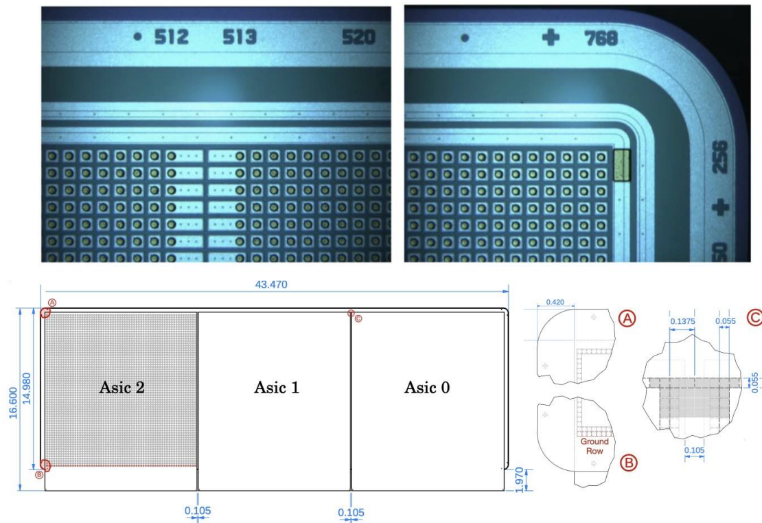
Figure 10. Top left: microscope image showing the elongated sensor pixels above the inter-ASIC region. Top right: image highlighting the ion-etched round corner of the sensor. Bottom: schematic of the sensor tile, showing the overall dimensions of the sensor and ASIC. The pixel layout is shown only under ASIC 2. There are 256 \times 256 active bonded pixels (only every fourth pixel is shown in the figure). An additional row of pixels identified in dark red provides a connection between the ASIC ground and the innermost guard ring of the sensor. Three corners, encircled in red, are shown in detail on the left (A, B, C).
