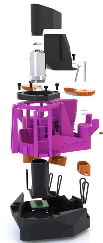
Figure 1. An exploded view of the OpenFlexure Microscope version 6.1.5, reproduced from [1] under the CC-BY-SA licence.
