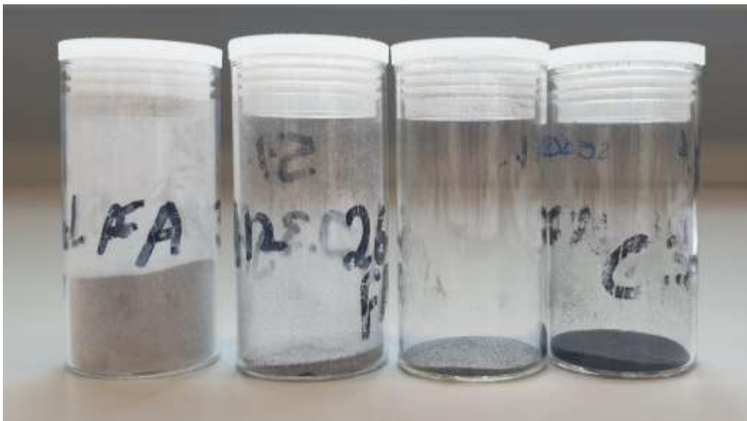
Figure 6.1.1: PA-12/FA blends (left to right) 1, 5, 10 and 20 wt.% FA.
