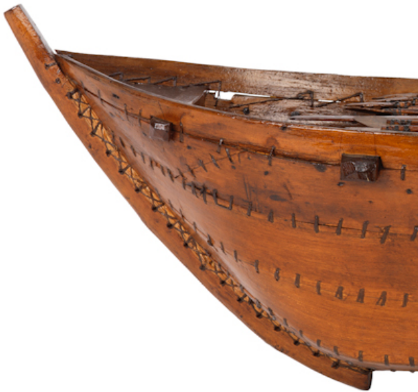
Figure 5: This close-up of a masula model held in the National Maritime Museum illustrates the way in which the planks were 'sewn' together. No nails were used to attach the planks to each other or internal fittings. NMM AAE0176.
