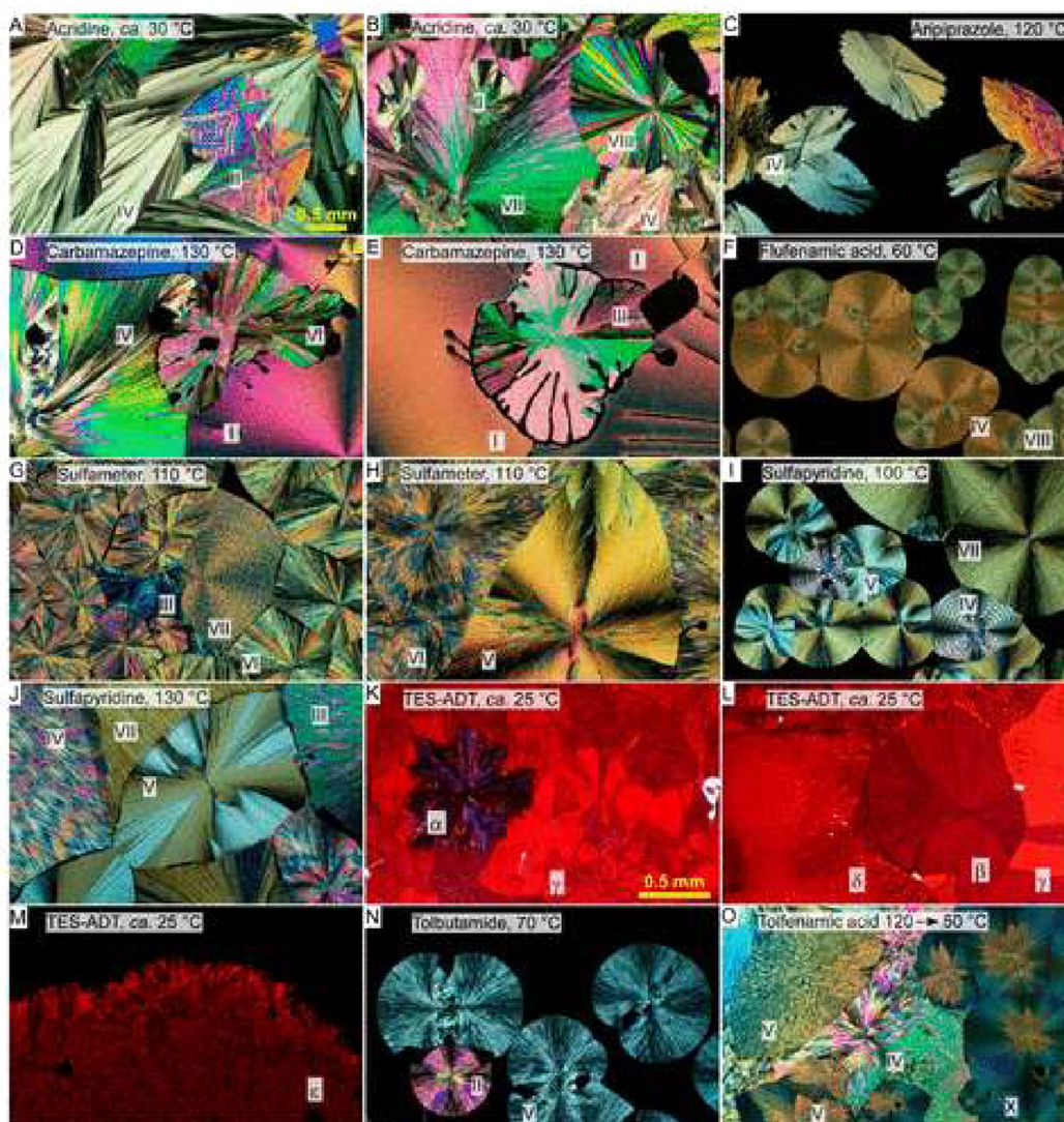
Figure 11. Polarized optical micrographs of melt-grown solid forms. CBZ is shown in E. Reproduced from reference 49. Copyright 2022 American Chemical Society.
