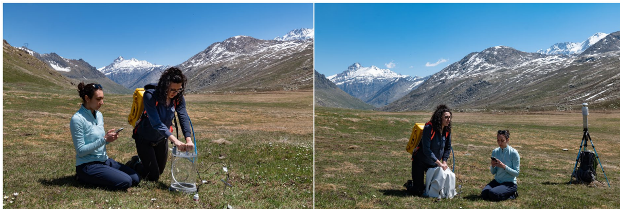
Fig. 4 Measurement procedure. The standard measurement cycle consists of two consecutive measurements at each point. The first measurement is conducted under natural light conditions using the transparent chamber (left) to determine the NEE. The second measurement is performed using the shaded chamber (right) to determine the ER. All individuals in figures have provided explicit consent for their images to be openly published.
