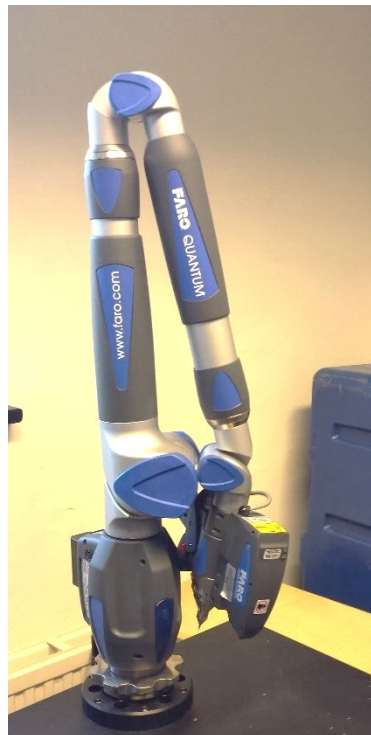
Figure 2.7: Image of 3D FARO QUANTUM ARM scanner
