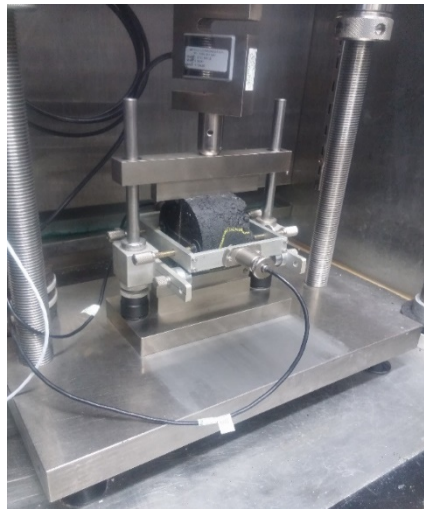
Fig. 3: Set-up for indirect tensile stiffness modulus test.
