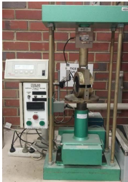
Fig. 1: Set-up for stability and flow tests.
