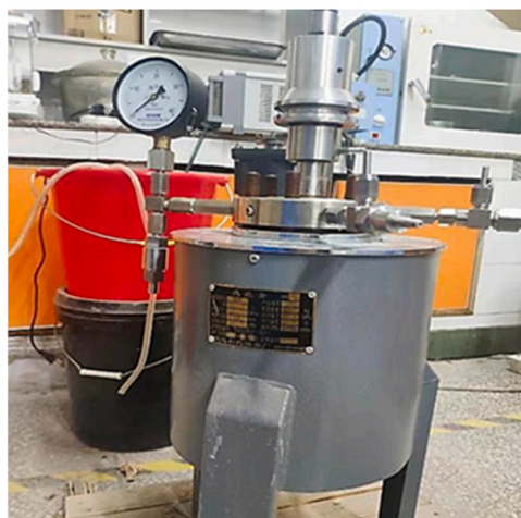
Fig. 1. The diagram of dynamic hydrothermal reactor (GCF).
