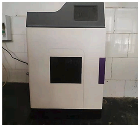
Fig. 2. The diagram of microwave digestion apparatus (ATPIO-24 T).
