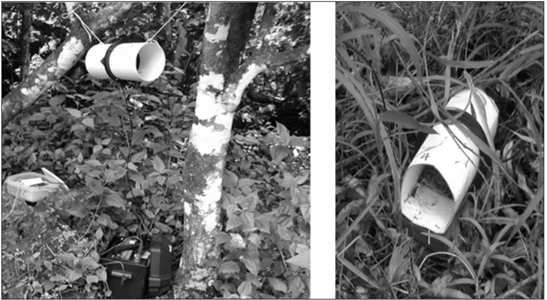
Figure 4. Brown treesnake ( Boiga irregularis ) bait delivery station hung from a tree (left) used on Guam, Northern Mariana Islands (1999–2000) and ground-placed mongoose ( Urva auropunctata : Syn. Herpestes auropunctatus ) bait delivery station (right) with PIT tag hoop antenna mounted in the center of the stations, Hawai'i Island, Hawai'i, USA (2007).
