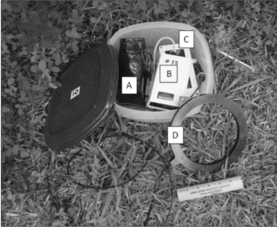
Figure 3. Automatic monitoring system components enclosed in weather-proof container—12 volts direct current compact sealed lead acid battery (A), data logger (B), AVID PIT tag reader (C), and trailing PIT tag hoop antenna (D used for monitoring bait station visitation by brown treesnakes ( Boiga irregularis ) on Andersen Air Force Base, Guam, Northern Mariana Islands (1999–2000) and mongooses ( Urva auropunctata : Syn. Herpestes auropunctatus ) on Hawai'i Island, Hawai'i, USA (2007). Note: label (10) on plastic container cover denotes device identification number.
