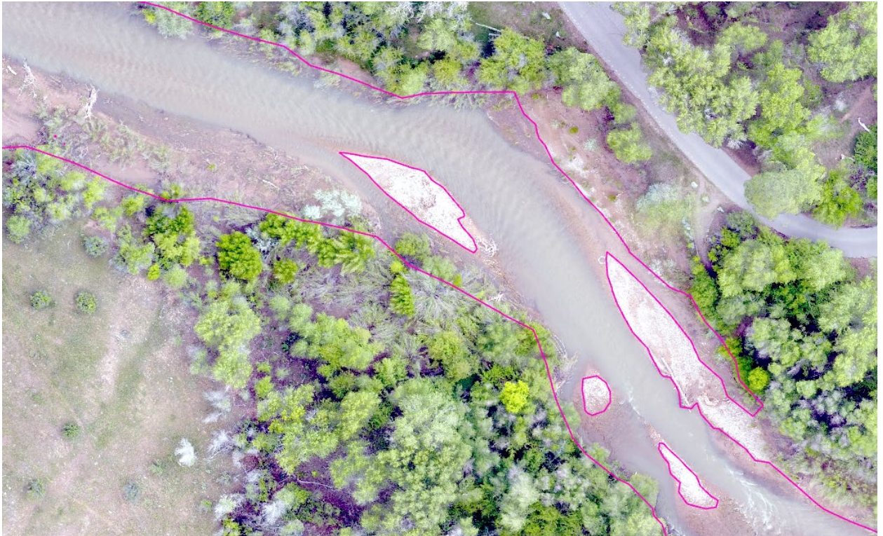
Figure 5: An Example Polygon/Polyline from the Manual Water Surface Delineation Overlaying USU Imagery, Diamond Fork River 06/09/23.
