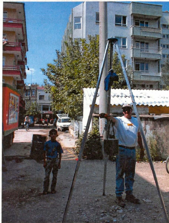
Figure 3.2 Photograph of the aluminum tripod and 90-kilogram weight used for 16- and 32-meter receiver spacings.
