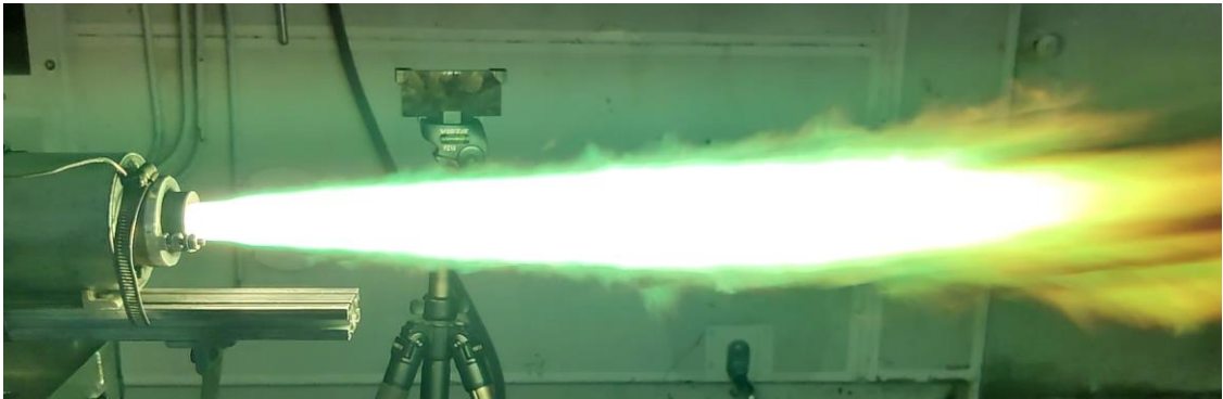
Figure 50: Green Exhaust Indicating Vaporized Copper. 0s < T < 1s .
