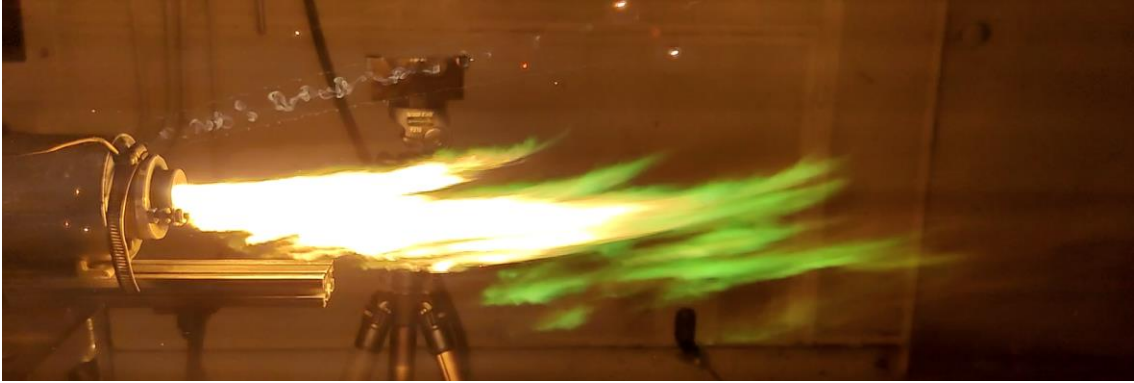
Figure 51: Motor Burnthrough with Debris
