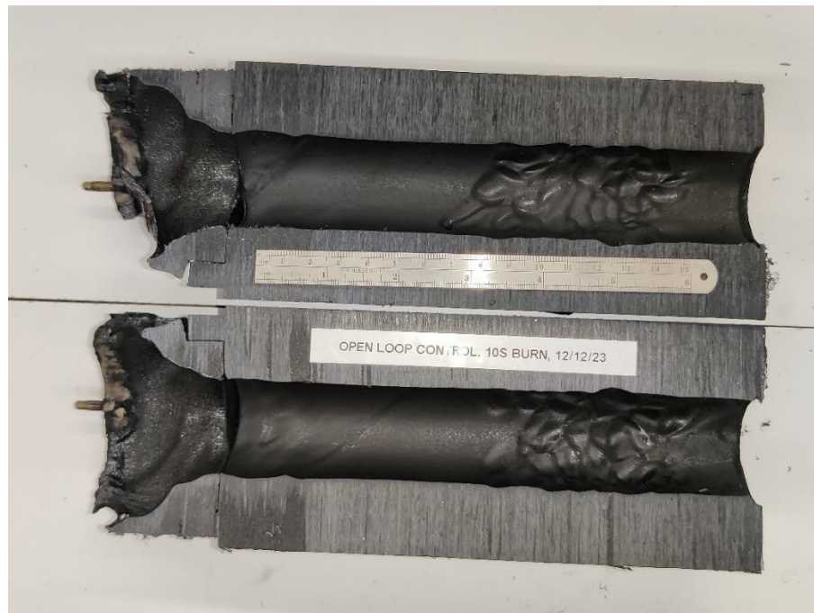
Figure 36: Burn 12, Fuel Grain Cross Section
