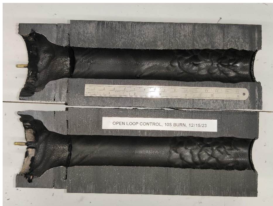
Figure 42: Burn 14, Fuel Grain Profile Cross-Section, Target O/F=3.5
