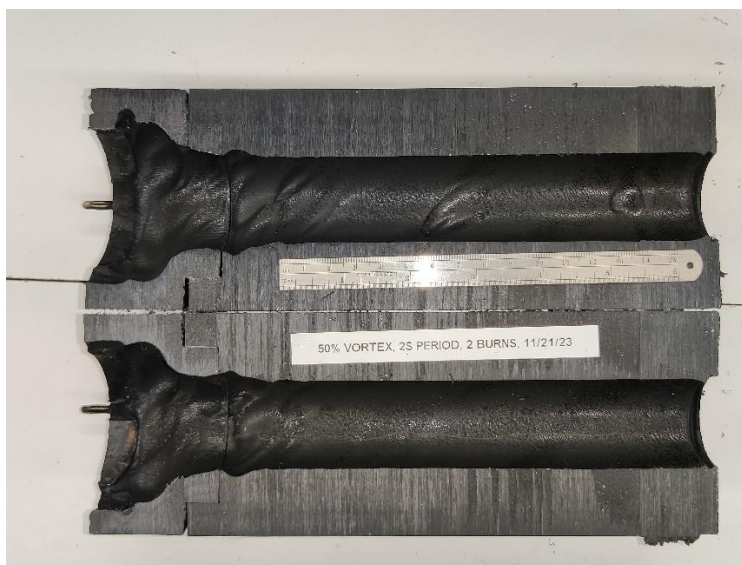
Figure 32: Burns 9 and 10 Fuel Grain Cross Section
