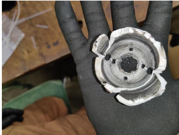
Figure 56: Post-Test Shattered Alumina 960 Dispersion Ring
