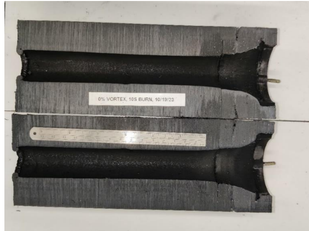
Figure 25: Axial Characterization Burn Fuel Grain Cross-Section
