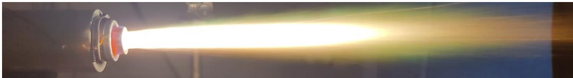
Figure 22: Axial Characterization Burn Exhaust Plume
