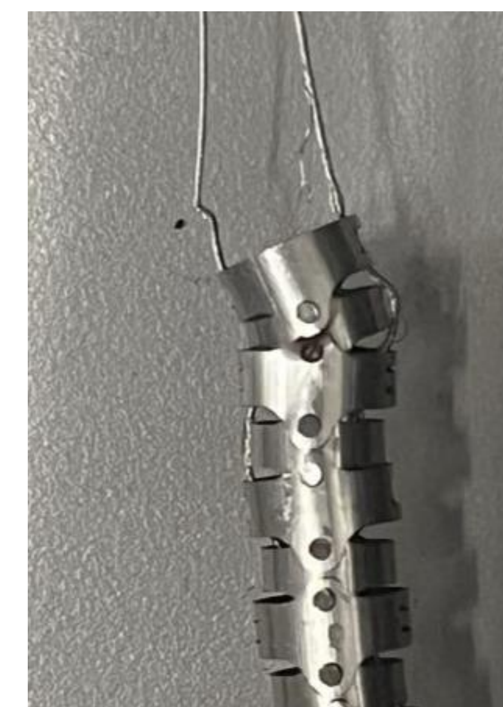
Figure 5: Damage incurred by backbone from compression testing
