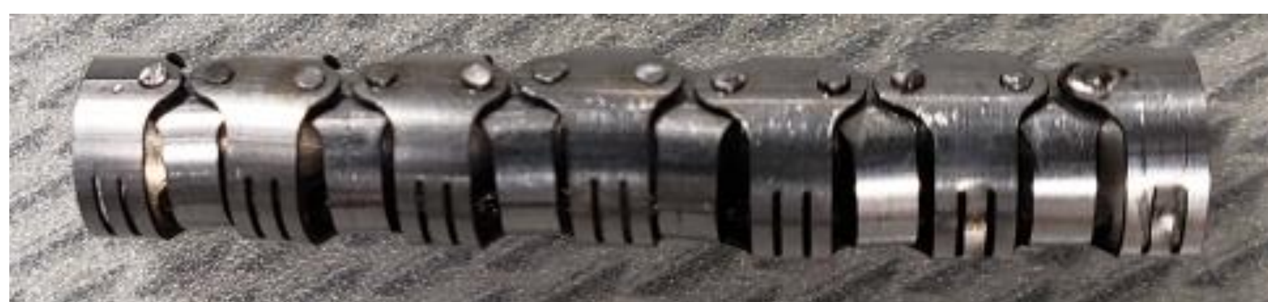
Figure 1: Final backbone laser cut from stainless-steel tubing
