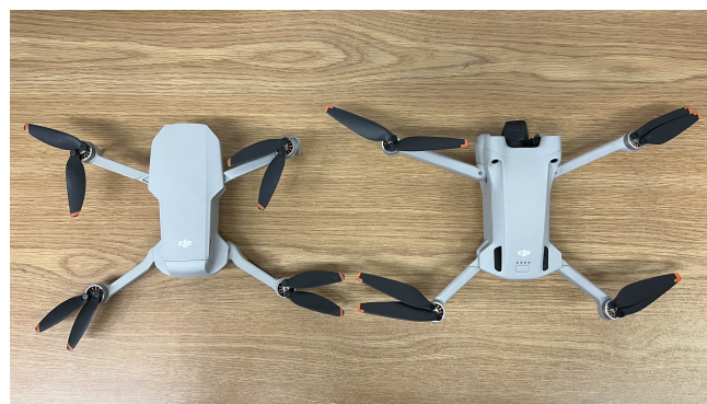
Figure 6. Drones used for aerial imaging. From left to right: DJI Mini SE and DJI Mini 3 Pro.
