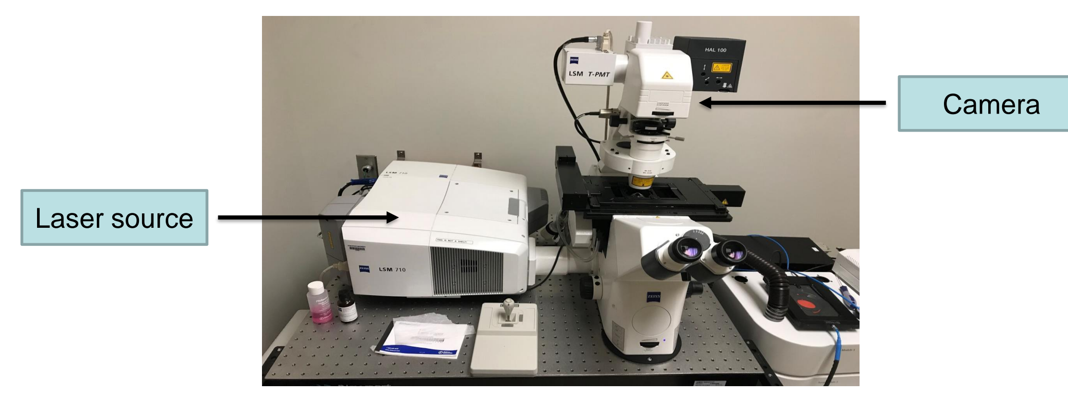
A Zeiss confocal microscope for taking fluorescence images
