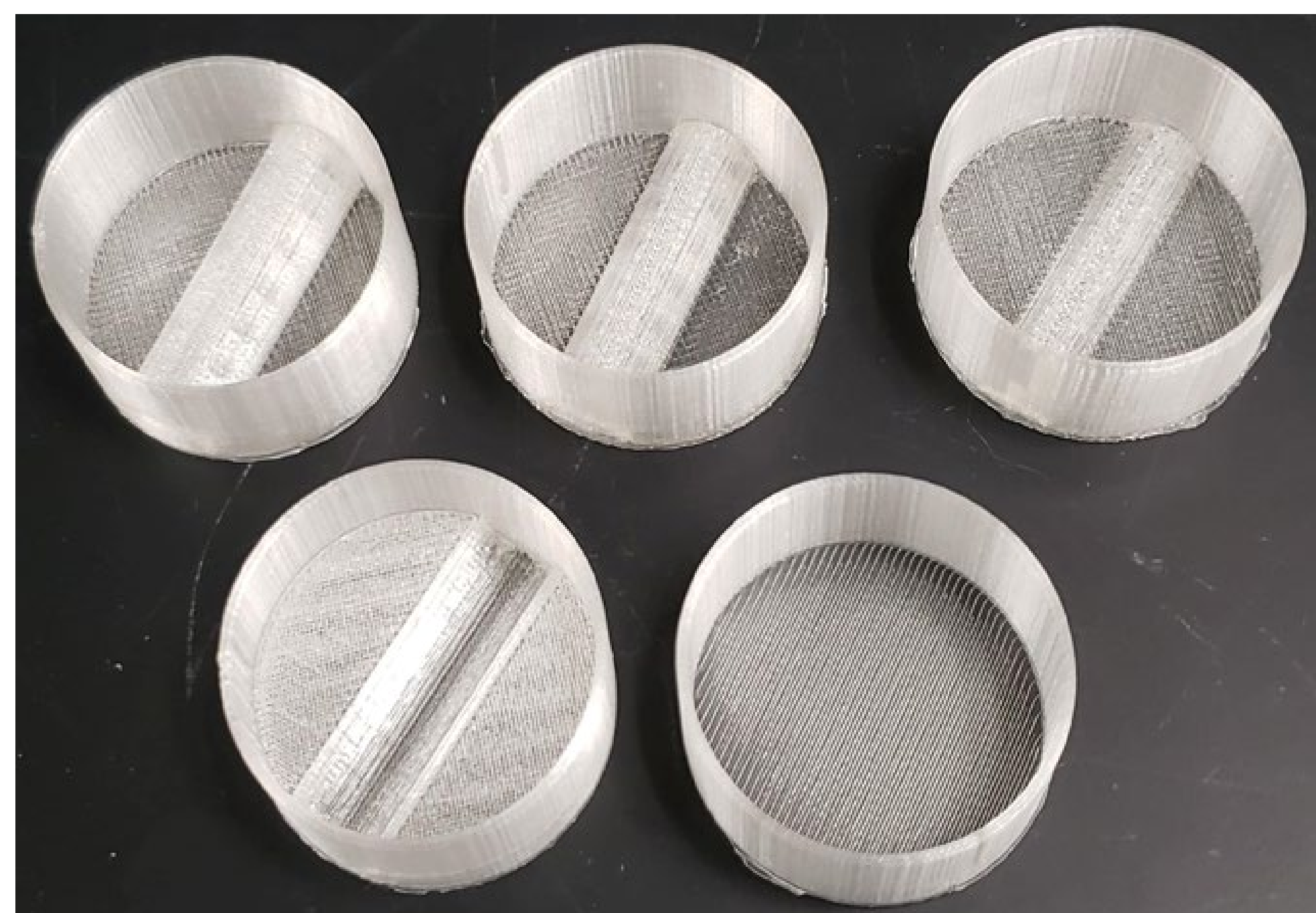
Figure 2 – PLA 3D printed scaffolds. (Top, from left to right) Large diameter convex, medium diameter convex, and small diameter convex. (Bottom, from left to right) concave, flat
