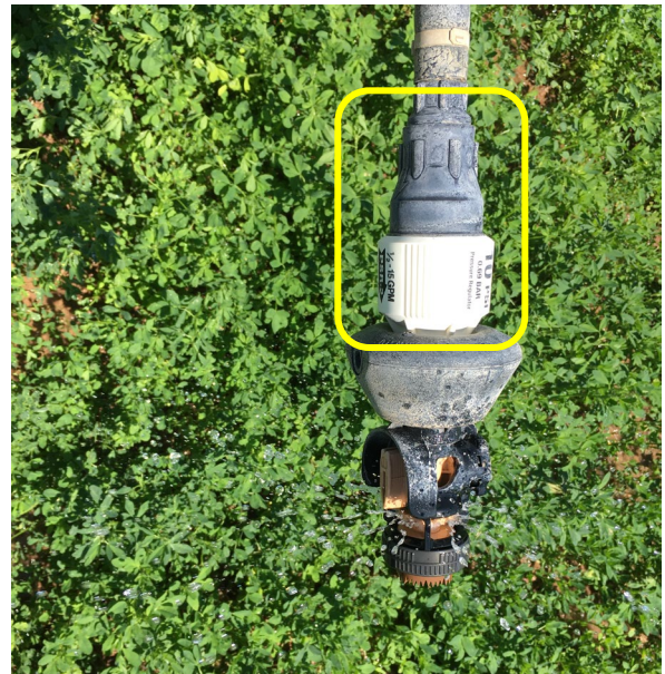
Figure 7. Center Pivot Sprinkler With a Pressure Regulator (in yellow box)
