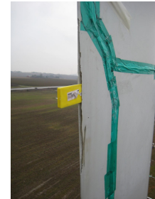
Figure 3. Image of damage introduced to V27 wind turbine blade.
