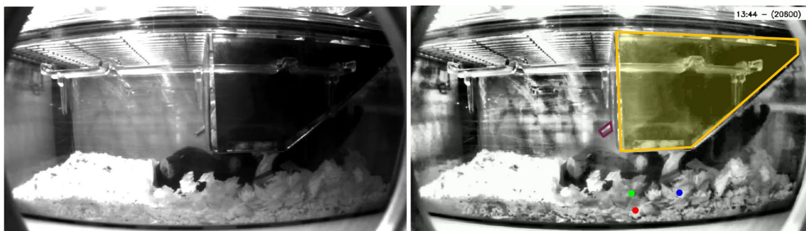
Fig. 1 An example video frame from our data, showing the raw video (left) and an enhanced visual (right) using CLAHE (Zuiderveld, 1994). In the latter, the hopper is marked in yellow and the water spout in pur-
