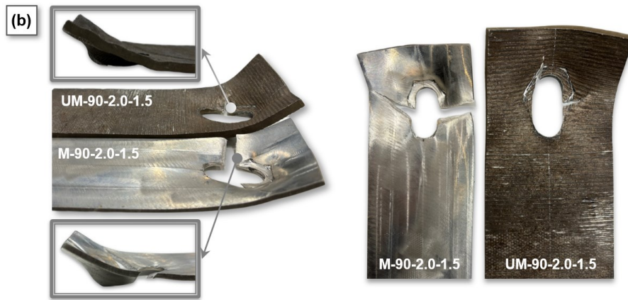
Fig. 9 Localized tearing failure: (a). Load-displacement curves; (b). Photos of specimens failed in LTF pattern.
