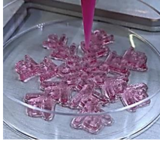
Fig. 11. A demonstration of a flower pattern created through DIW printing using aloe vera/cellulose nanofibrils bio-hydrogel ink [28].
