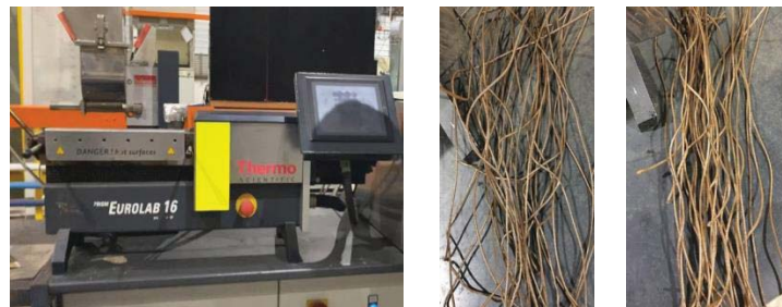
Figure 1. A wired-shaped product is produced by mixing sieved kenaf, PP granules, and MAPP granules.
