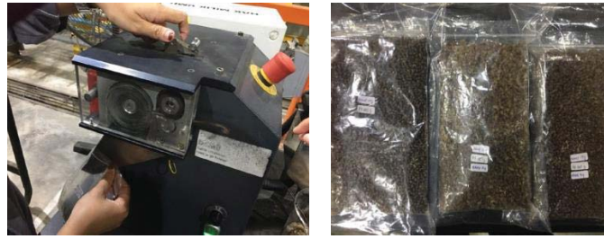
Figure 2. A pelletizer machine is used to cut wired-shaped composite into pellets form.
