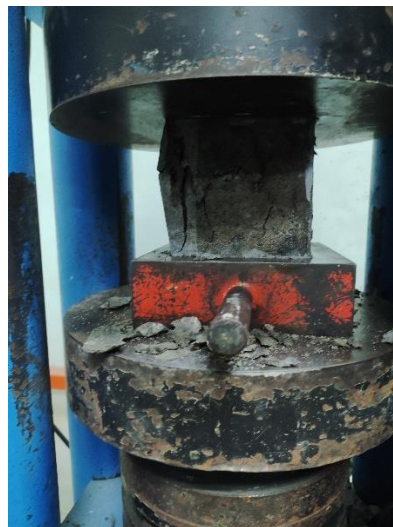
Figure 6.4: Compressive strength test
