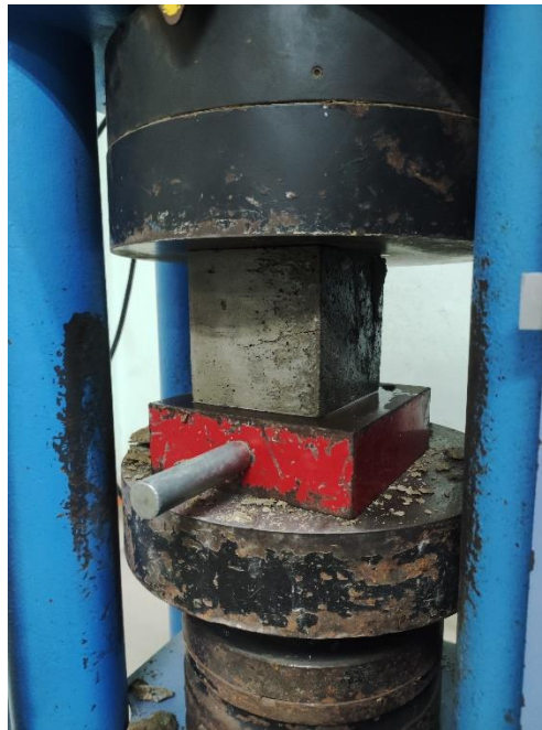
Figure 6.3: Compressive strength test of 0% concrete
