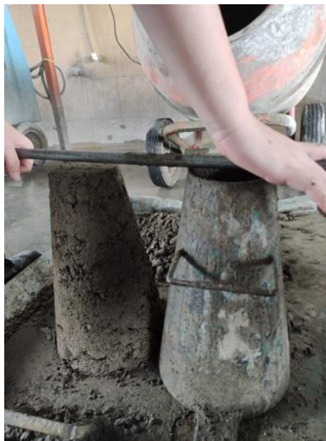
Figure 6.2: Slump test of 4% coconut ash concrete
