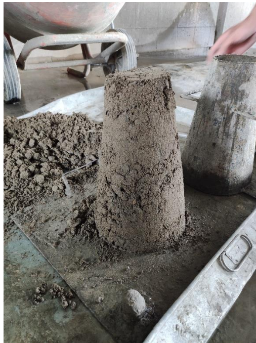
Figure 6.1: Slump test of 0% concrete
