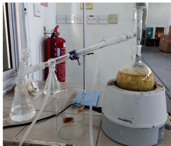
Fig. 1. Hydro distillation extraction apparatus set up.
