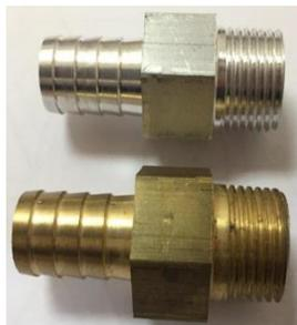
Figure 2. Actual case study product with hole depth 55.00mm.
