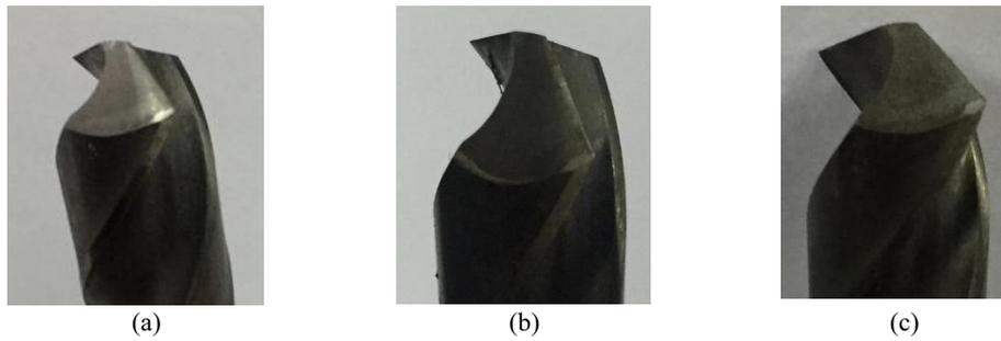
Figure 4. The drill cutting tool conditions after the drilling process. (a) Diameter 10.00 mm; (b) Diameter 13.00 mm, and (c) Diameter 14.50 mm.
