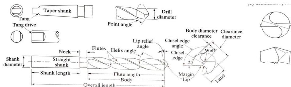
Figure 1. Twist drill part name [4].
