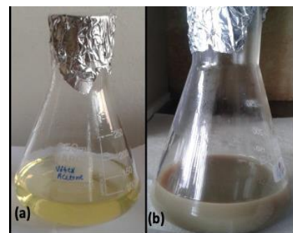
Figure 4 Synthesis of silver nanoparticle of V. negundo (a) plant extract with AgNO 3 (b) synthesized nanoparticles.
